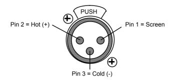
Fig 2.6.3: Pin arrangement for XLR inputs on the SPX20
